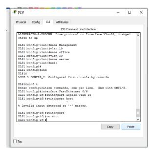
Repeat this configuration for interface fa0/18 on DLS2 and ALS1, and then verify the switchports on DLS1, DLS2 and ALS1 are members of VLAN 10.
