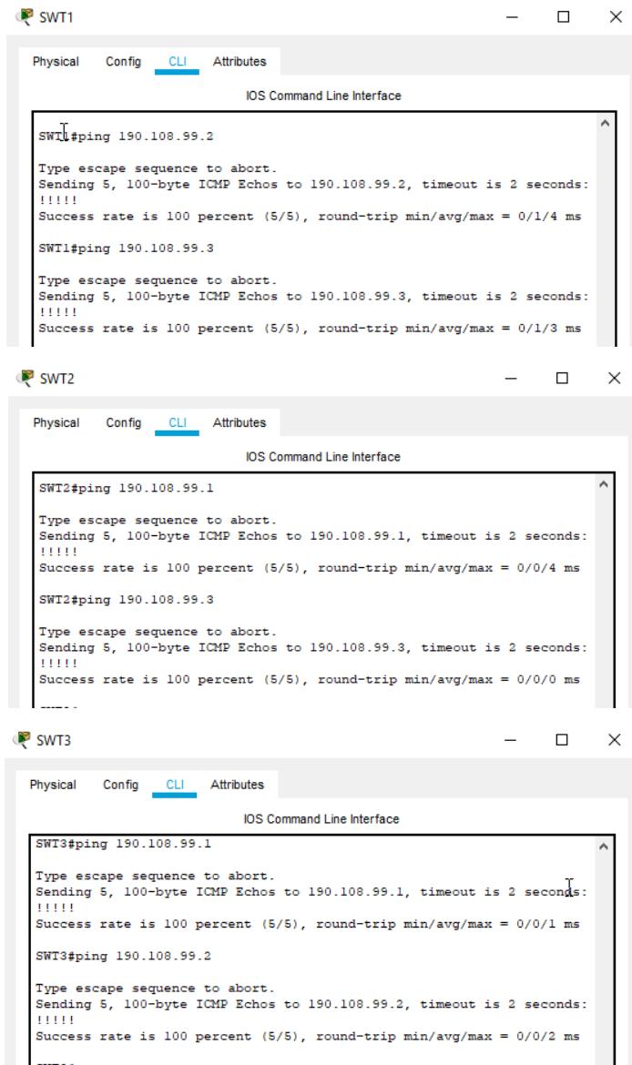
The image displays three separate terminal windows, each representing a different switch (SWT1, SWT2, and SWT3). Each window shows the CLI interface with the 'CLI' tab selected. The windows are titled 'SWT1', 'SWT2', and 'SWT3' respectively. Each window contains a command-line interface window with the title 'IOS Command Line Interface'. Inside these windows, the user has run the 'ping' command to test connectivity between switches. The output for each ping command is as follows:
