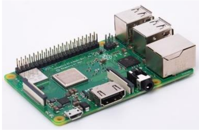
Figura 8. Raspberry pi 3 B+. Recuperado de: raspberrypi.org
