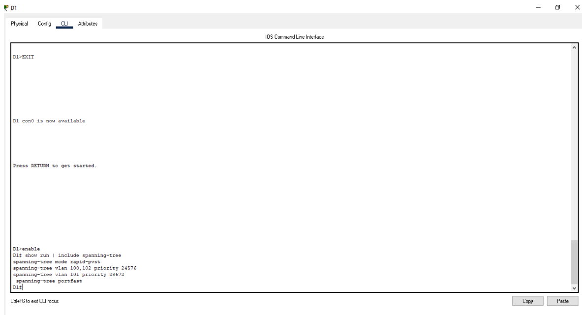
Figura 5. aplicando show run | include spanning-tree en D1
