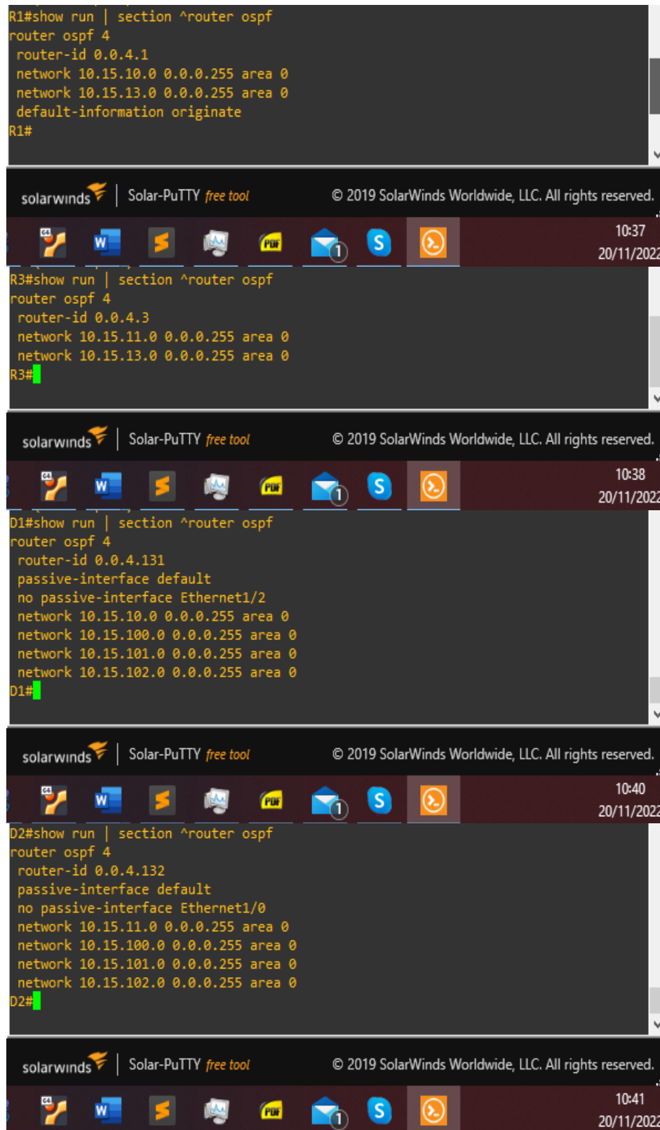
Figura 10: Verificación de show run | section ^router ospf on R1, R3, D1, and D2
