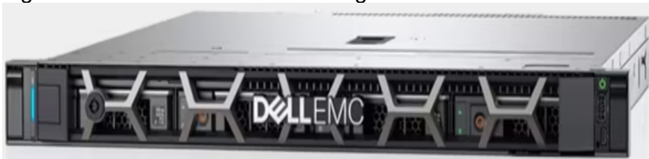
Figura 8. Servidor en rack PowerEdge R250
