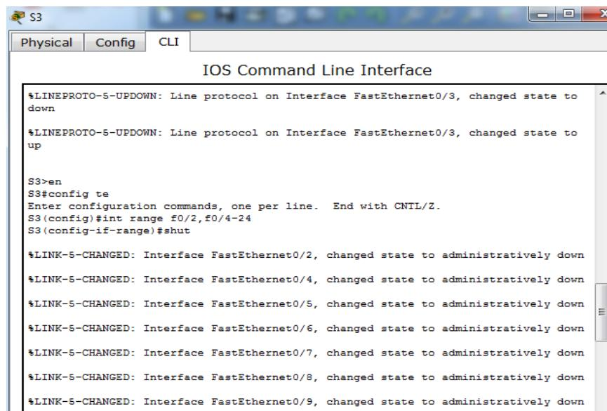
The screenshot shows the Cisco IOS CLI interface for router S3. The window title is "S3". The tabs at the top are "Physical", "Config" (which is selected), and "CLI". The main area displays the command output:
