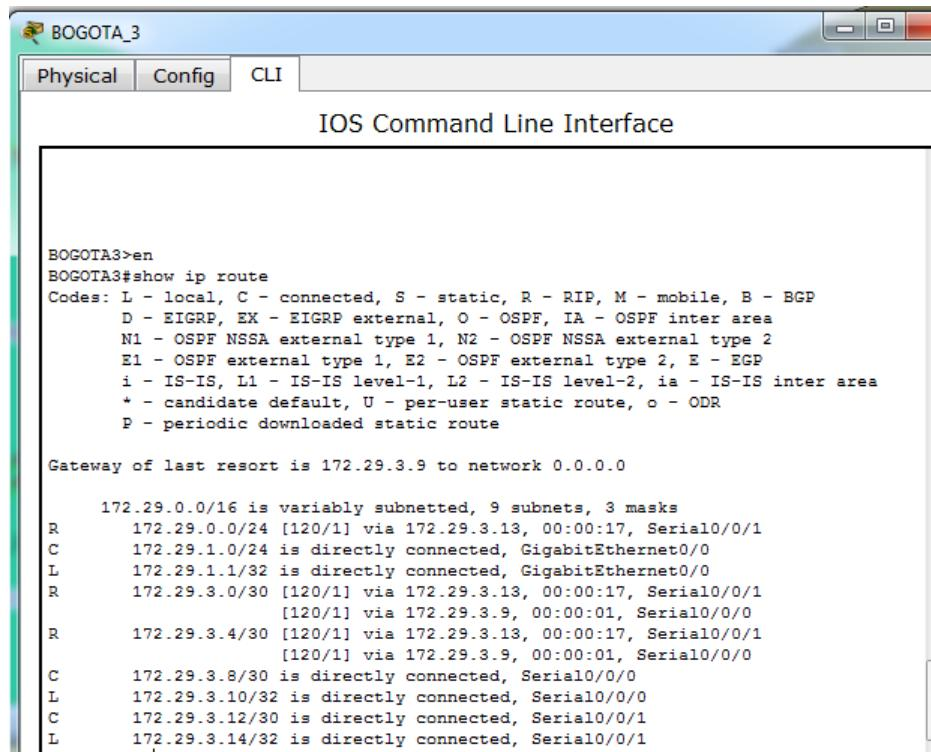
The screenshot shows the CLI interface for router BOGOTA3. The window title is "BOGOTA\_3". Below the title bar are tabs for "Physical", "Config", and "CLI", with "CLI" being the active tab. The main area displays the output of the "show ip route" command.
