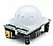
This motion sensor module uses the LH0778 Passive Infrared Sensor and the BSS500B1 IC to control how motion is detected.
