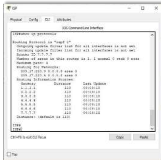
Figura 40. Show ip route protocols en Router ISP.
