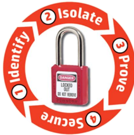
Figura 1-2-1 Principio de aislamiento. (Allen-Bradly. By Rockwell Automation.)
