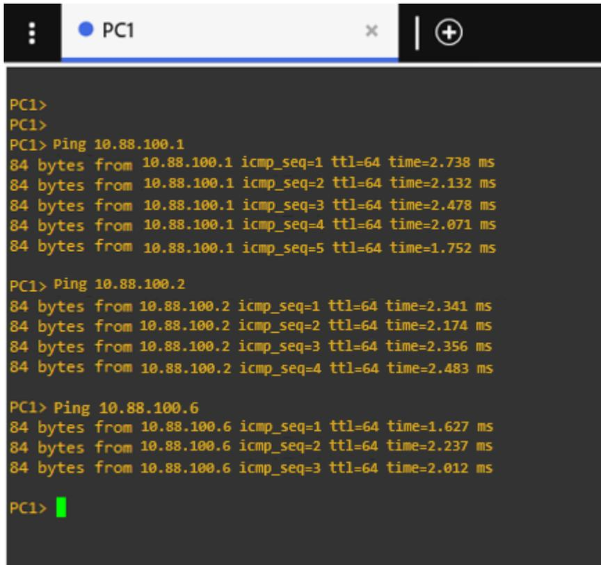
A screenshot of a terminal window titled 'PC1'. The terminal shows the execution of three ping commands. The first command is 'Ping 10.88.100.1', which results in five successful responses with varying times. The second command is 'Ping 10.88.100.2', resulting in four successful responses. The third command is 'Ping 10.88.100.6', resulting in three successful responses. The terminal ends with a green cursor on the 'PC1>' prompt.
