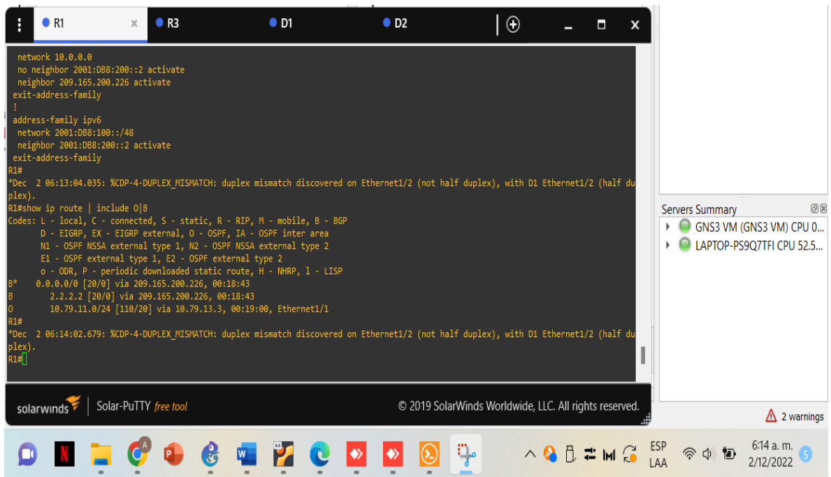
Figura 56. Show ip route | include O/B R1
