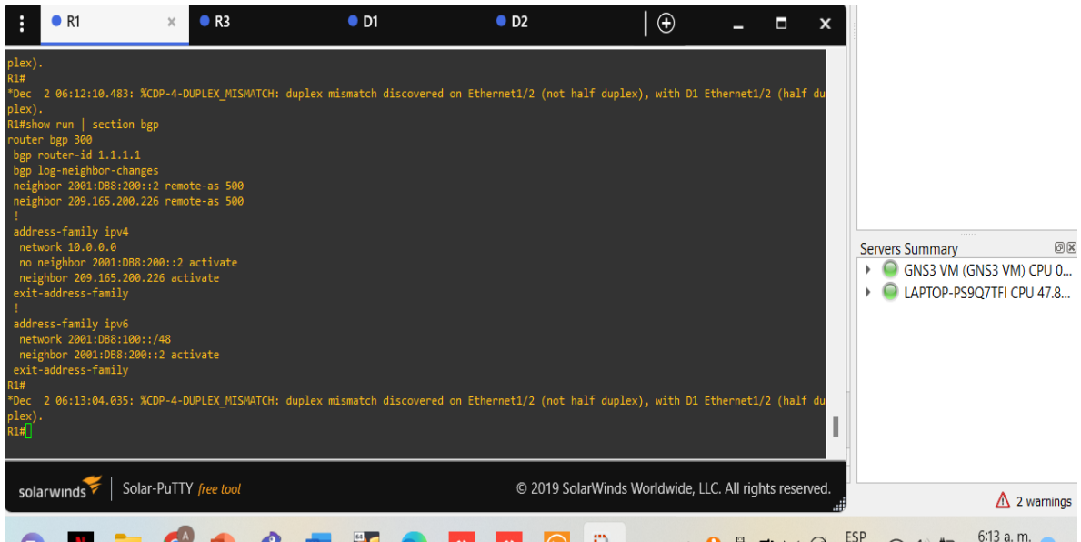
Figura 55. Show run | section bgp R1
