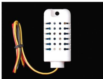
AM2302/DHT22 with big case and wires
