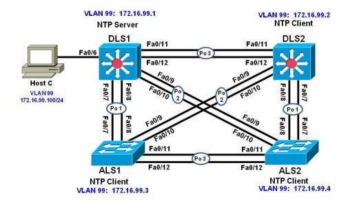
All Switch-to-Switch connections are 802.1q trunks
