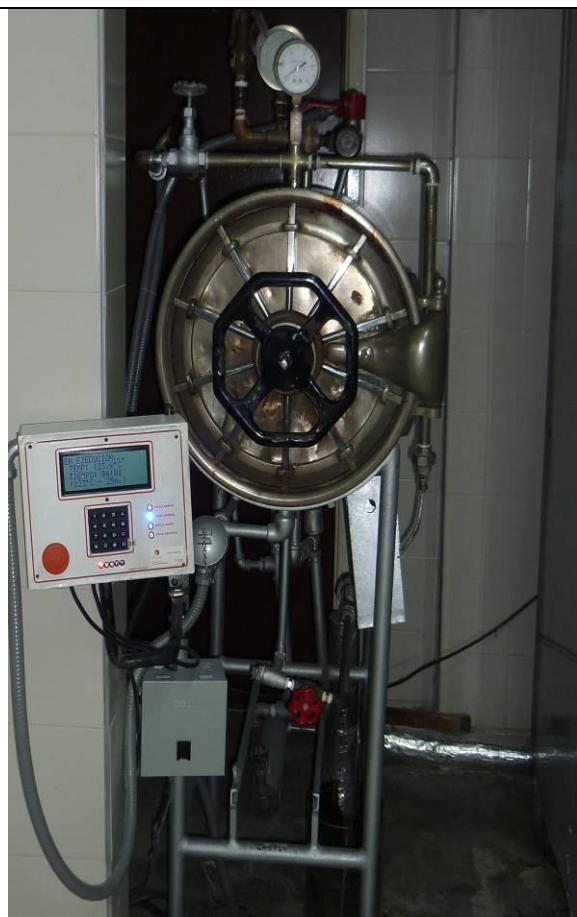
Figura No 8. Autoclave – Sunclave del Hospital Departamental Tomas Uribe Uribe E.S.E
