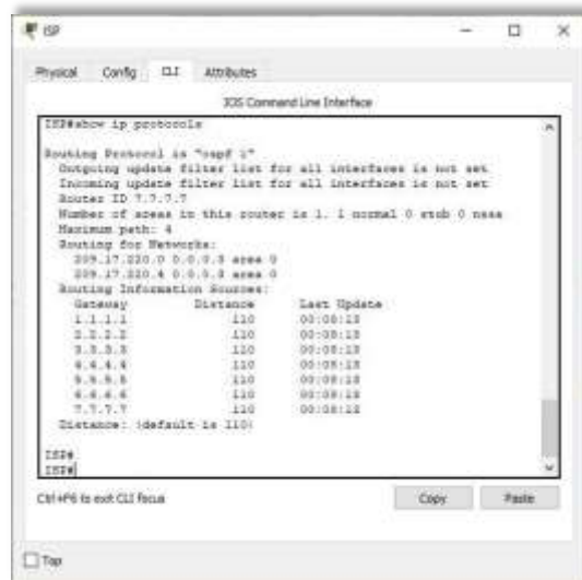
Figura 40. Show ip route protocols en Router ISP.
